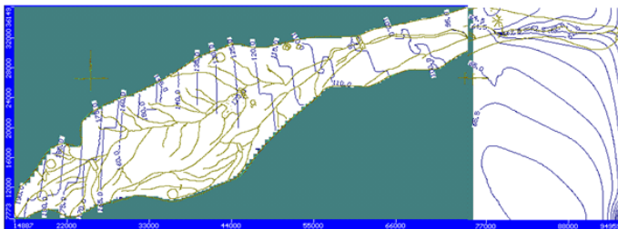
Figure 9 Base case water table condition in middle layer after 10 days
