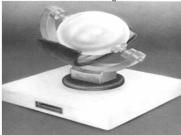
Fig 2: Campell-Stokes sunshine recorder used to measure sunshine hours at Eldoret meteorological station.
