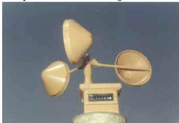
Fig 1: Cup-type anemometer used to measure wind speeds at Eldoret meteorological station.
