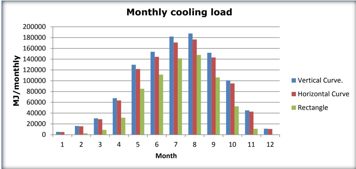
Figure 3:- monthly cooling load without glazing area.
