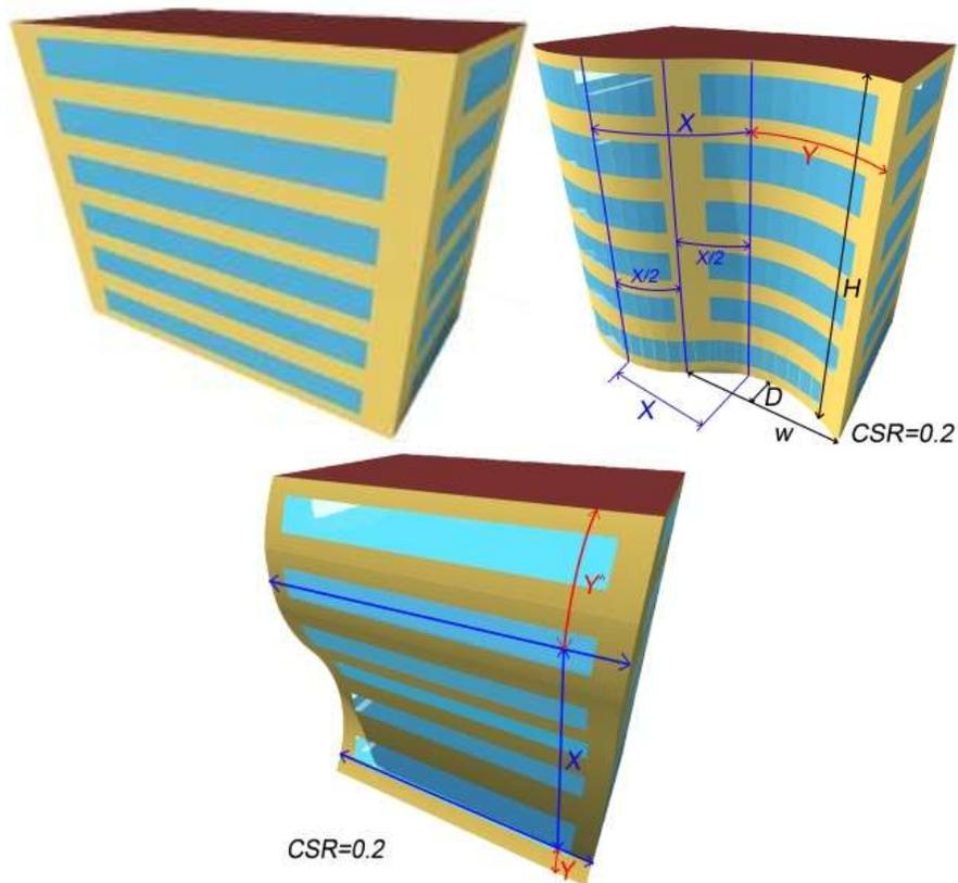
Figure 5:- Adding glazing area according to glazing to floor area ratio.
