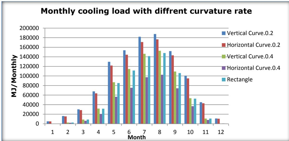
Figure 9:- Comparing monthly cooling load after increasing curvature rate.
