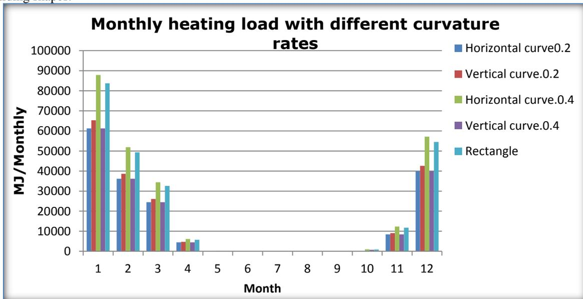
Figure 10:- Comparing monthly heating load after increasing curvature rates
