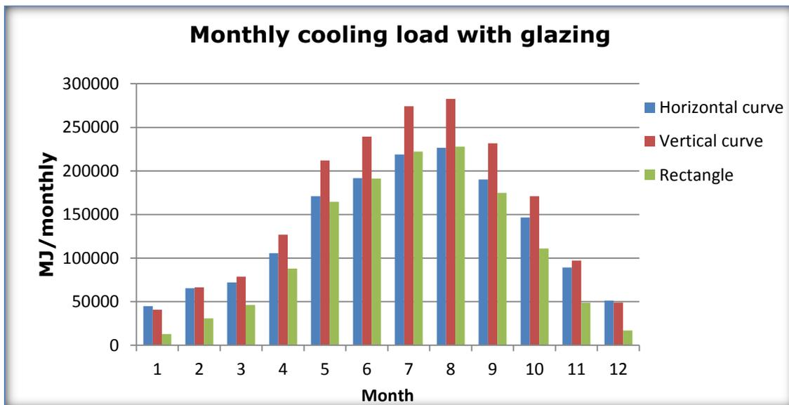
Figure 6:- monthly cooling load after adding glazing area.
