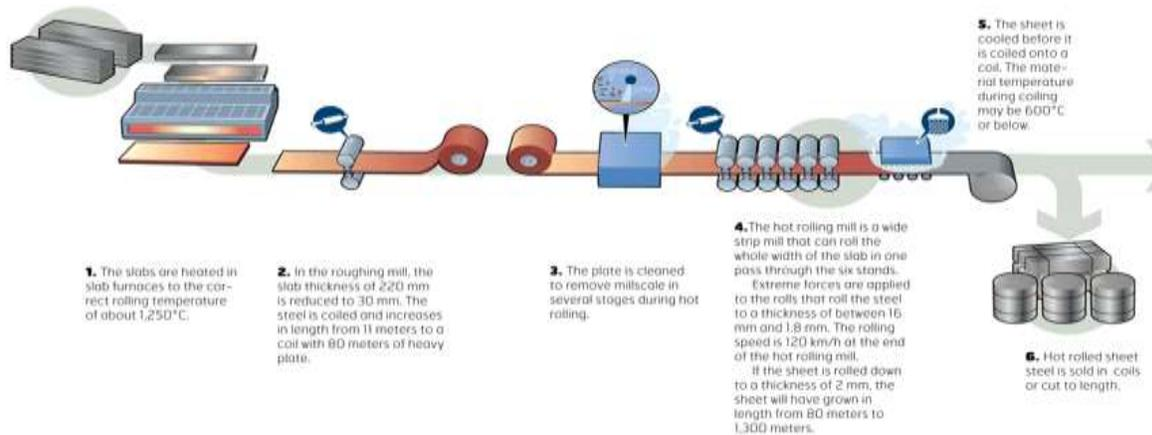
**Fig. 1:-** Schematic representation of Hot Rolling Mill.
