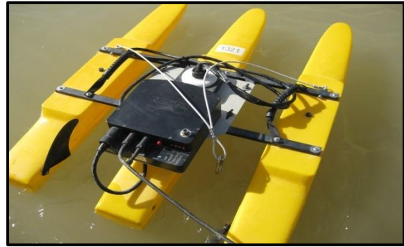
Fig.3: SonTek river surveyor ADCP
