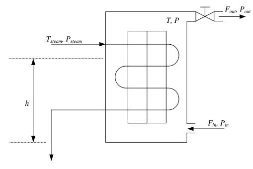
Figure 1. A schematic diagram of an evaporator
