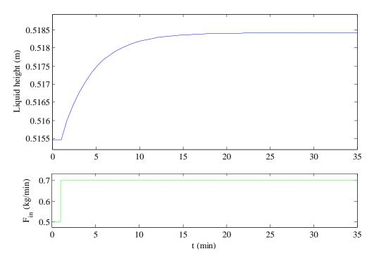
Figure 5. Dynamic response of liquid height to a +0.2 kg/min step change in feed flow rate
