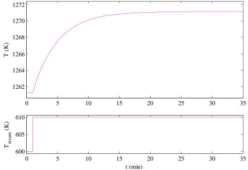
Figure 8. Dynamic response of system temperature to a +10 K step change in steam temperature
