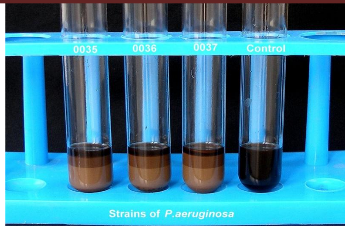
Fig.2. Emulsification Stability Test for the three bacterial strains of Pseudomonas sp.
