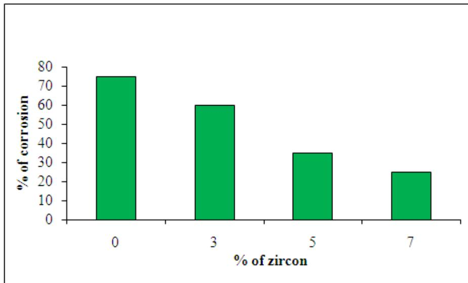
**Figure 81:-** Percentage of corrosion of Al 7075/zircon composites for 72 hours of exposure time
