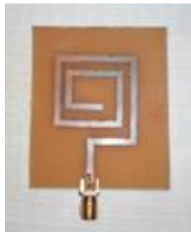
Fig. A.17, The fabricated antenna
