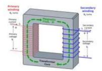
The direction of the magnetic field produced by a coil can be determined by the right hand grip rule. If the fingers of the right hand are wrapped around the magnetic core of a coil in the direction of conventional current through the wire, the thumb will point in the direction the magnetic field lines pass through the coil.
