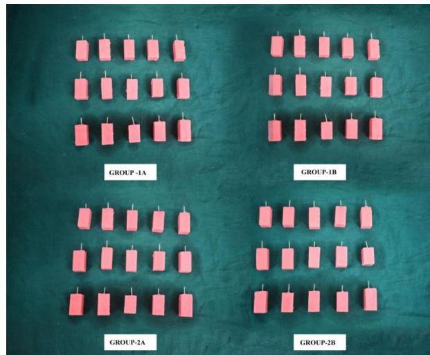
Figure 8:- Specimen mounted on acrylic blocks and grouped as 1a, 1b, 2a, 2b based on the post space diameters and resin cements.
