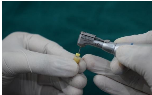
Figure 4:- Post space preparation in the specimens.
