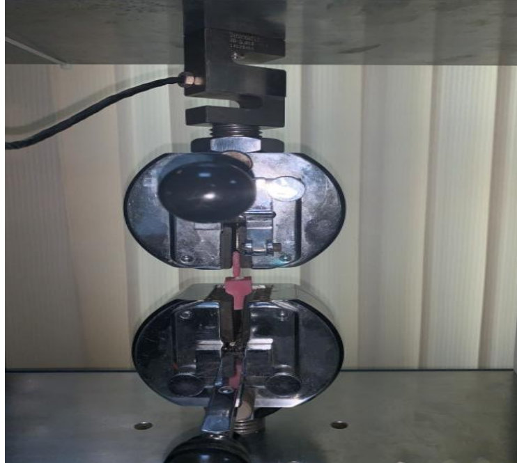
Figure 9:- Specimens mounted on universal testing machine for pullout test.
