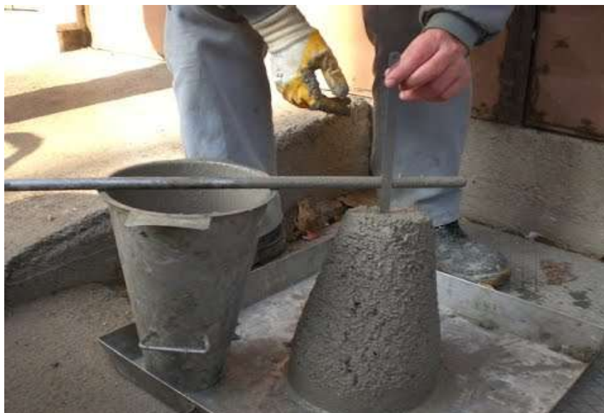
Fig- 18:- Slump Cone Test.
