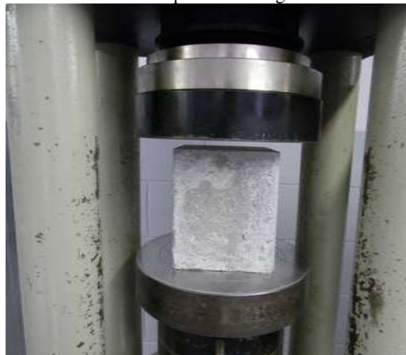
Fig-8:- Compressive Test On Cube.
