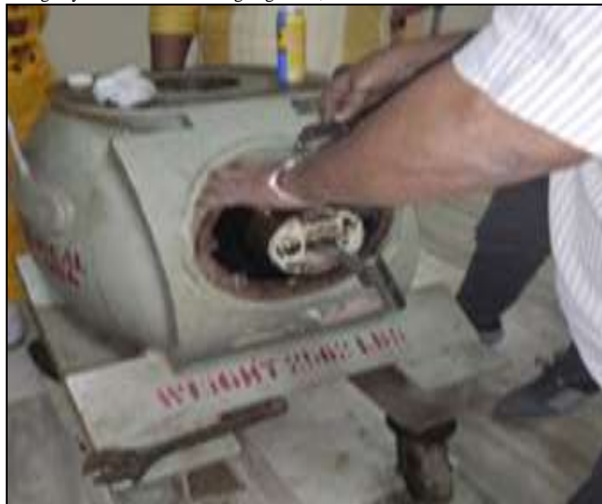
Fig. 2:- Lubrication of shielding container.
