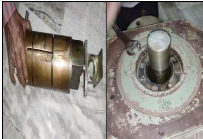
Fig. 4:- (a) Source drawer (b) T-handle.
