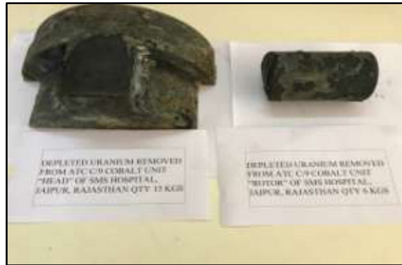
Fig. 5:- Depleted uranium removed from ATC C/9 Head Qty 15 Kgs and Qty 6kgs from Rotor.
