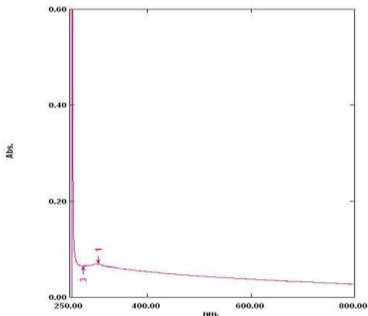
**Fig 2:-** UV-spectrum of synthesized HAP (using *Acalypha indica* leaf extract) Nanoparticle.
