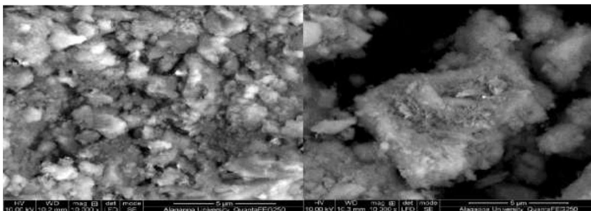
**Fig 8:-** FESEM image of HAP Nanoparticle synthesized using *Acalypha indica* leaf extract as solvent.
