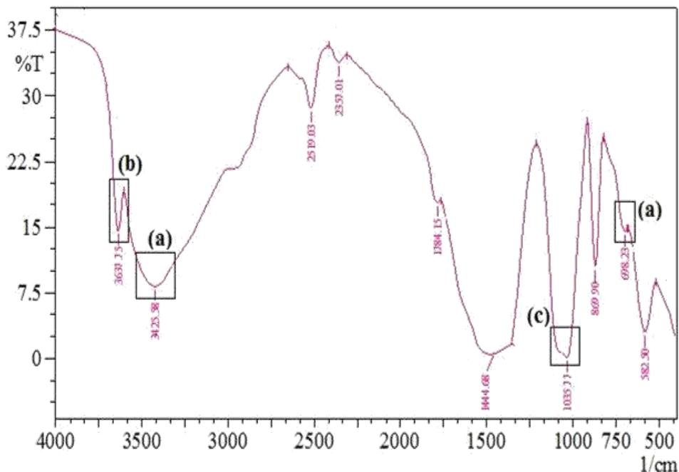
Figure 4:- FTIR Spectra of HAP using Acalypha indica extract as solvent.
