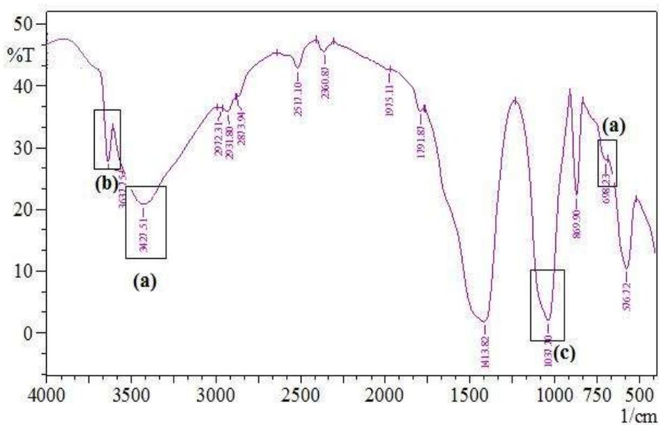
**Figure 3:-** FTIR Spectra of HAP using *Carica papaya* extract as solvent.
