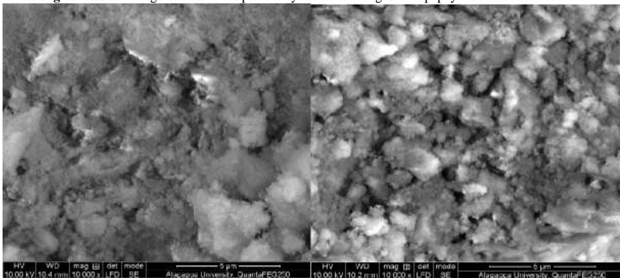
Figure 7, showed the FESEM micrograph of the sample synthesized HAP Nanoparticle (using *Carica papaya* leaf extract as solvent). The morphology of synthesized HAP Nanoparticle shows the agglomerated and resolved particle is represented in figure. the morphology of the particle seems to be spongy and agglomerated structure.
