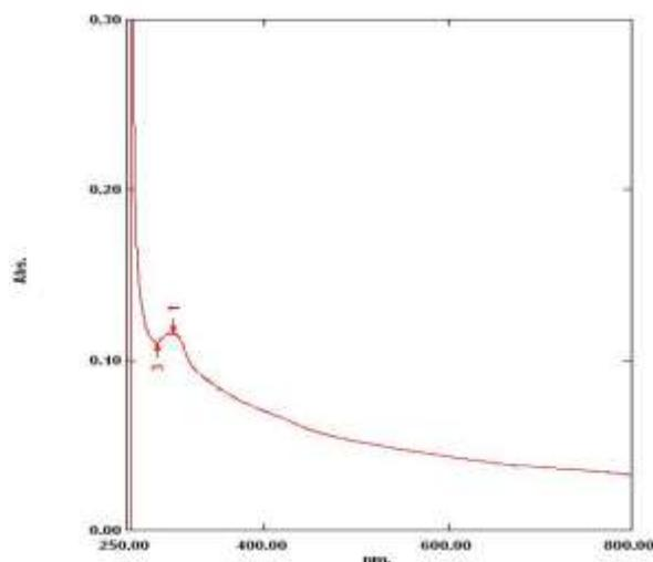
**Fig 1:-** UV-spectrum of synthesized HAP (using *Carica papaya* leaf extract) Nanoparticle.
