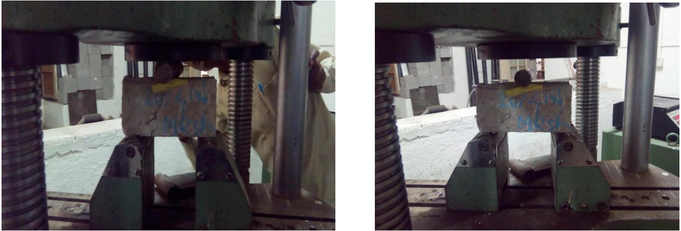
Fig.17 Flexural test arrangement
