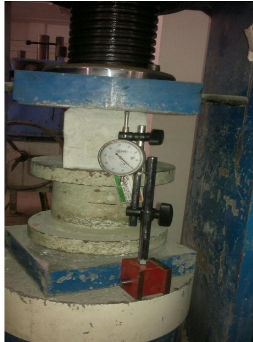
Fig.13 failure of block in Compression(left side), compressive testing apparatus setup(right side)
