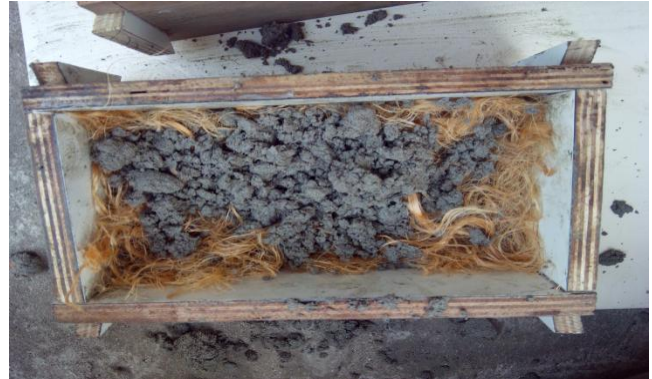
Fig.8 Fibers placed in a mould without being wetted in a geopolymeric paper slurry
