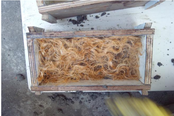
Fig.8 Fibers placed in a mould without being wetted in a geopolymeric paper slurry
