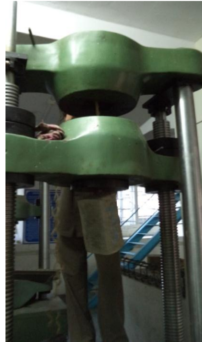
Fig.16 Bond test of ropes reinforced with geopolymeric paper blocks
