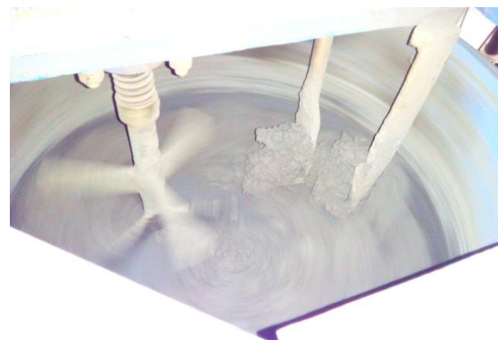
Fig. 3 Mixing of all the ingredients in rotating drum
