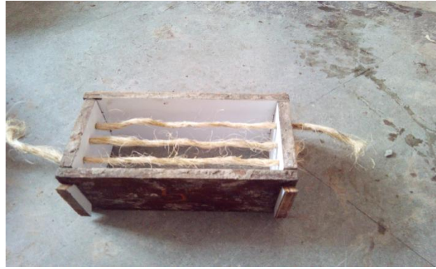
Fig.6 Strands inserted in the moulds throughout
