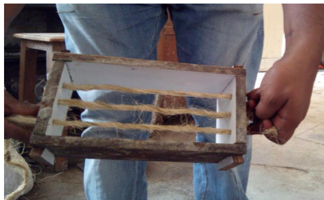
Fig.7 Strands Positioned in a mould throughout
