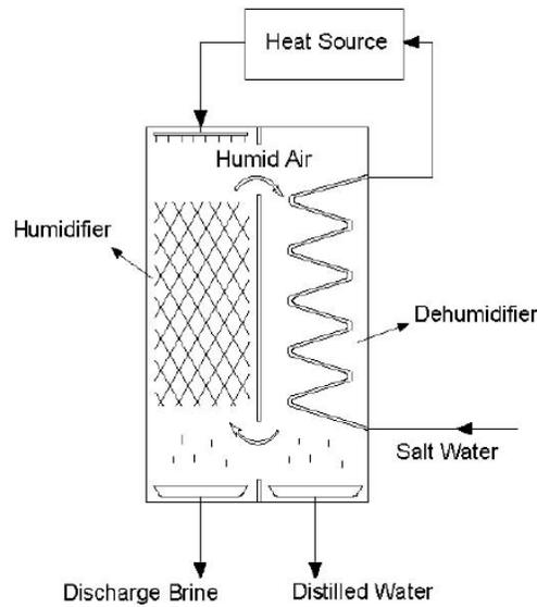
Figure 1 Principle of HD process[1]
