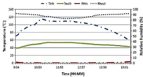
Figure 7 Effect of relative humidity of the air entering and exiting the humidifier[6]
