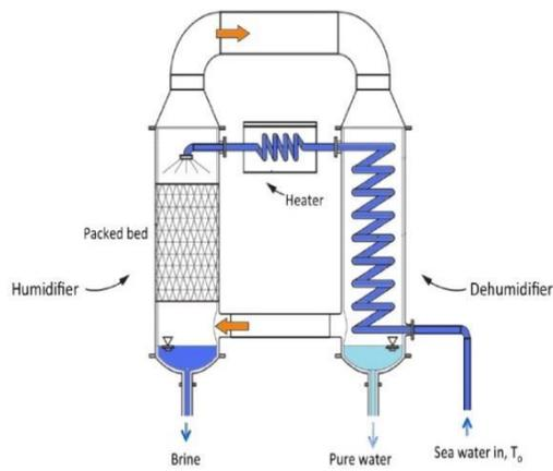
Figure 4 Closed Air-Open Water Cycle
