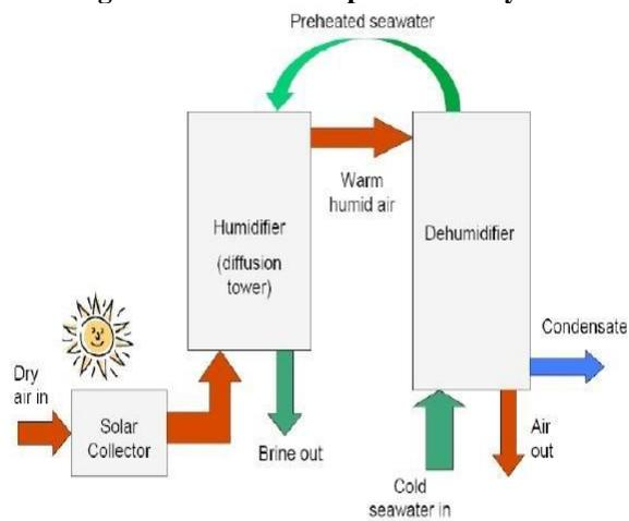
Figure 5 Air-heated Cycle
