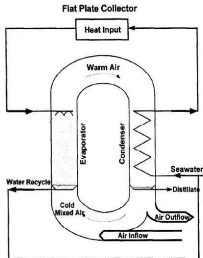
Figure 3 Closed Water-Open Air Cycle[4]
