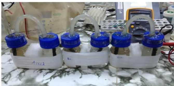
Figure (1): two-chambers of microbial fuel cell example of microbial fuel cell, cells producing electricity and biofilm formation
