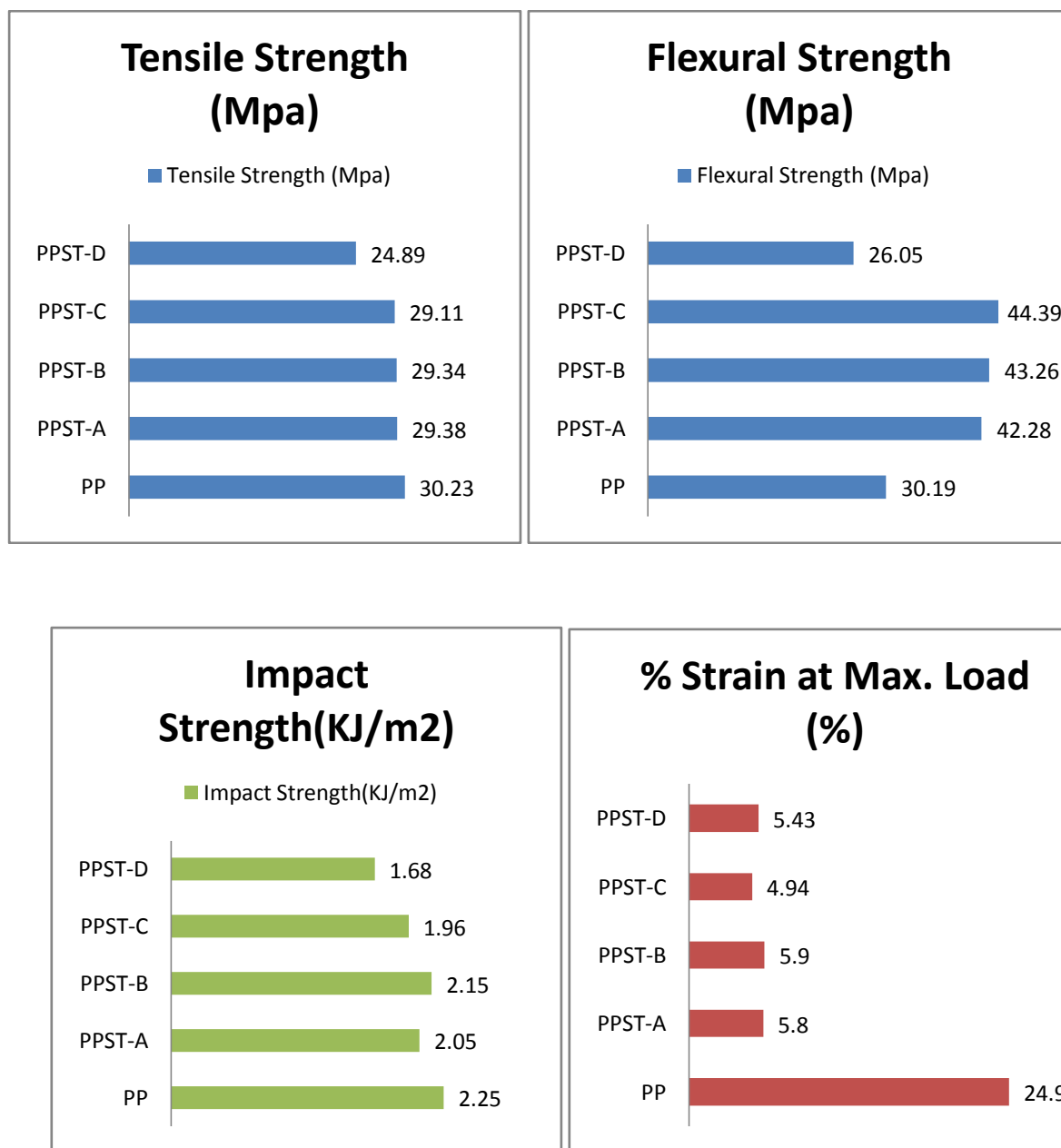
Figure no. 2: The tensile, flexural, impact and %strain of PP/Starch blend.
