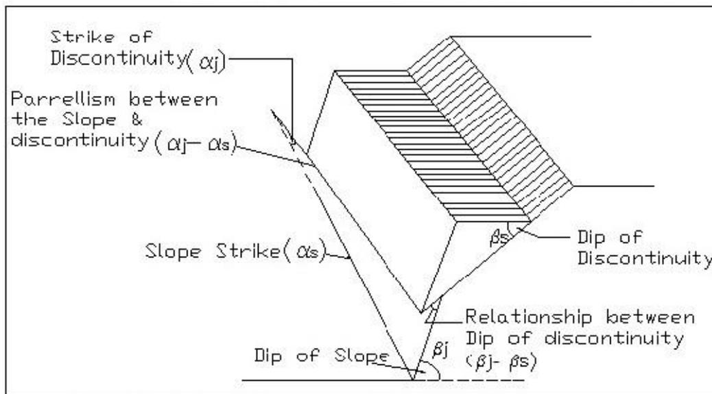
**Fig.6 Schematic diagram of Slope Mass Rating(SMR)**
