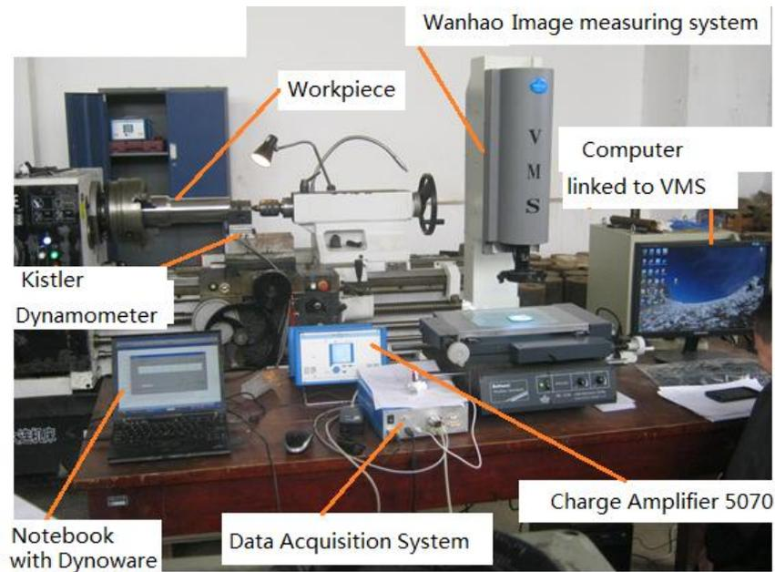
**Figure 1: Layout of the Equipment for Force Measurement and Tool Wear Measurement**
