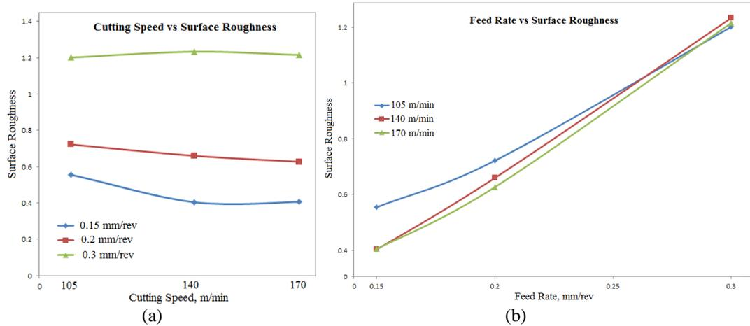
**Figure 3: (a) Cutting Speed and (b) Feed Rate vs. Surface Roughness of 42CrMo4**
