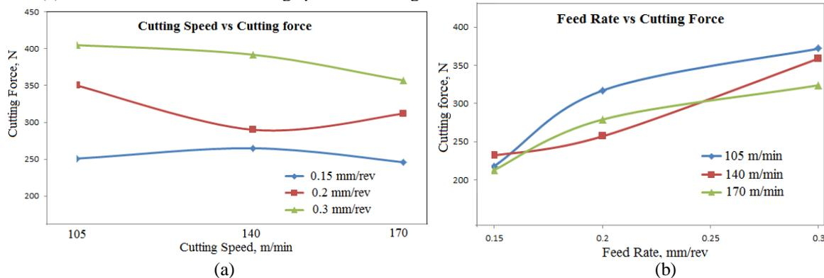
**Figure4: (a) Cutting Speed and (b) Feed Rate vs. Cutting Force of 42CrMo4**
