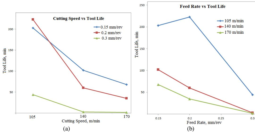
**Figure 2: (a) Cutting Speed (b) FeedRate vs. Tool Life of PCBN Tool Inserts**
