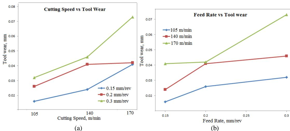
**Figure 5: (a) Cutting Speed and (b) Feed Rate vs. Tool Wear of PCBN**
