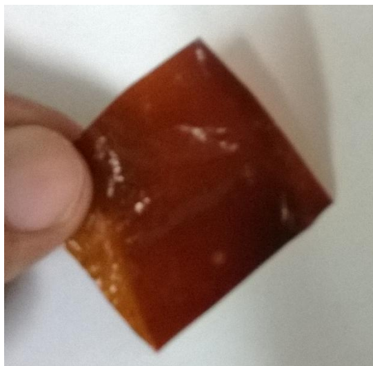
Fig.6. CMGG/Ag nanocomposites film
