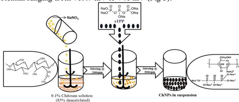
**Fig.1 Schematic representation of preparation of Chitosan nanoparticles by ionic gelation method**
