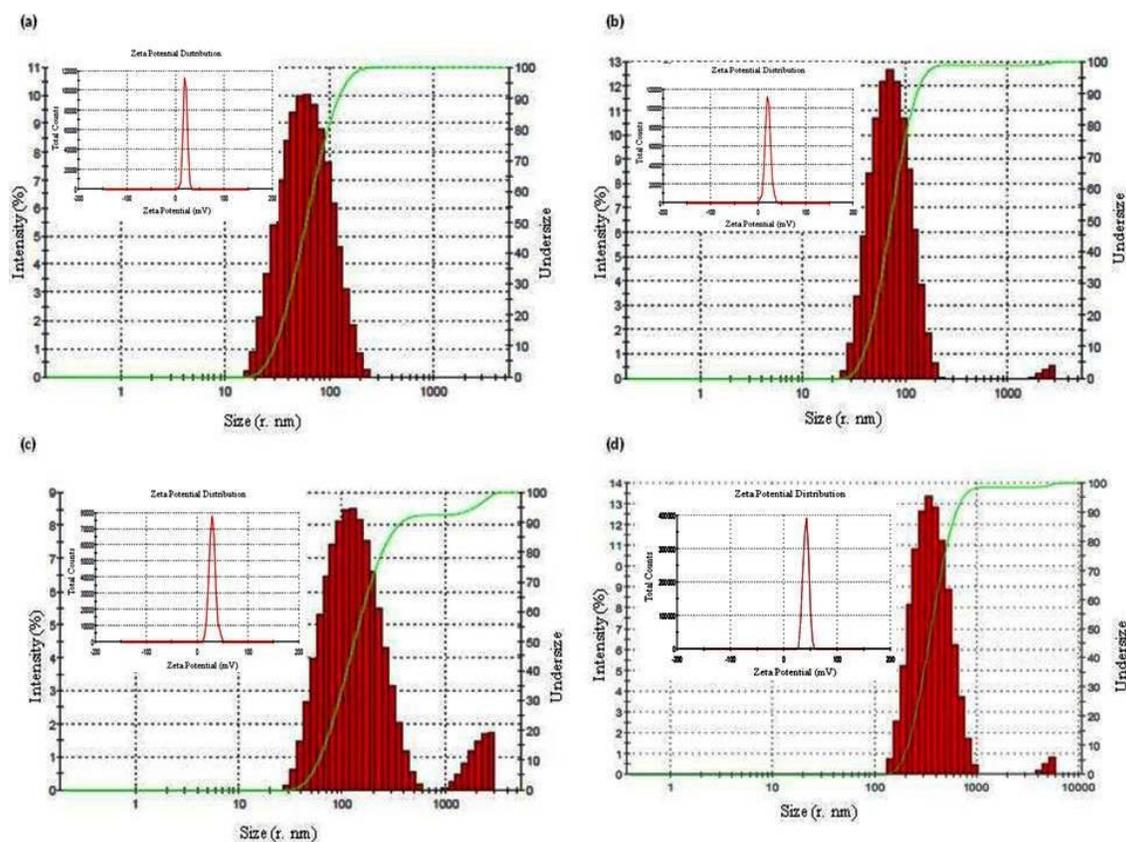
**Fig 2.** DLS measurements showing (a) mean diameter (51.97 nm) with polydispersity index 0.219 and  $\zeta = +19.7$  mV , (b) mean diameter (80 nm) with polydispersity index 0.213 and  $\zeta = +20$  mV, (c) mean diameter (111.4 nm) with polydispersity index 0.365 and  $\zeta = +29.3$  mV, and (d) mean diameter (245.9 nm) with polydispersity index 0.245 and  $\zeta = +41$  mV
