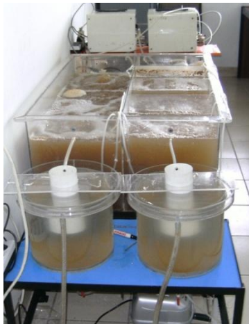
Figure 3:- A continuous step aeration reactor used for biodegradation assay of produced water
