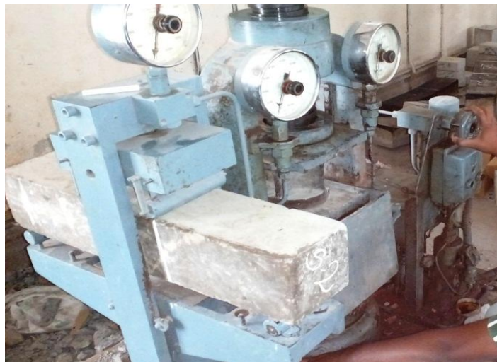
Fig 2:- Beam is set for testing.
