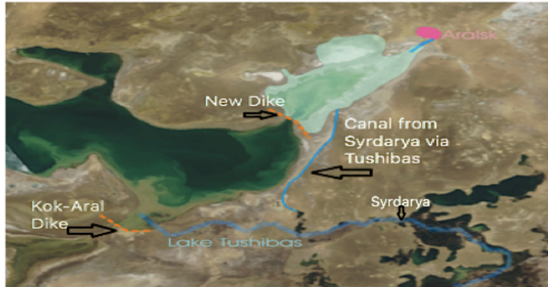
Figure 5:- Saryshiganak project area with dam (orange), supply canal and access canal to Aralskharbour (blue) and flooded area (transparent) Remark: The flooded area was taken from an bathymetric map which was not entirely exact as the satellite image shows (Phase 2)
