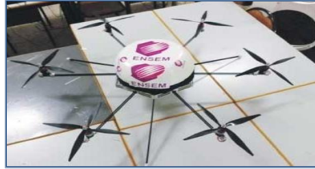
Figure 1:- A picture of the developed hexarotor (EAAS\ENSEM)
