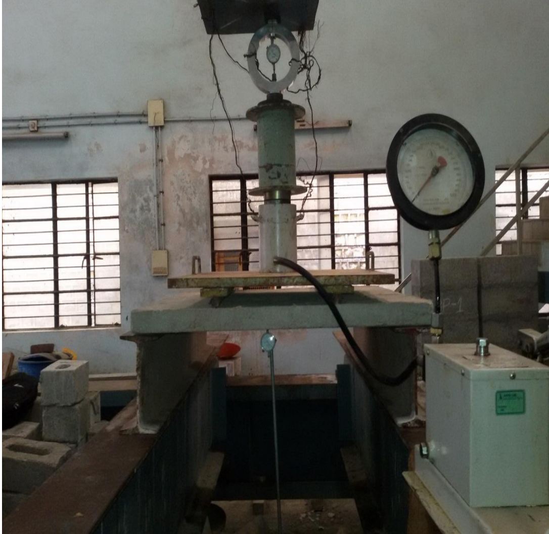
Fig 7:- Testing of slab specimens (structural lab)
