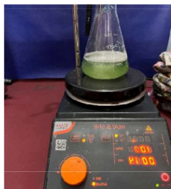
50 Figure 2. Schematic representation of the green synthesis of copper nanoparticles (CuNPs) using Cissus quadrangularis stem extract. Bioactive phytochemicals present in the extract act as natural reducing and stabilizing agents, facilitating the conversion of \text{Cu}^{2+} ions into stable copper nanoparticles under mild, eco-friendly conditions.
