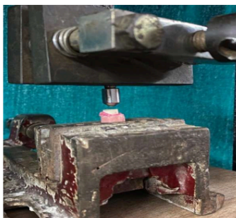
FIGURE 2- SAMPLE MOUNTED ON UNIVERSAL TESTING MACHINE
