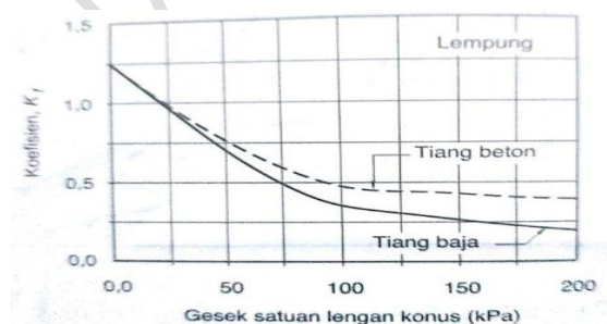
Figure 2-3 Kf coefficient in clay
