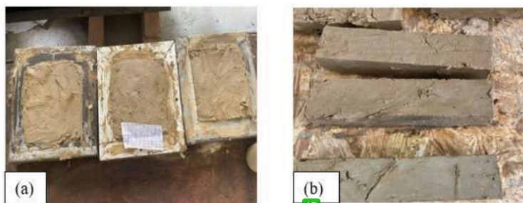
Figure 2: - Test pieces of 100 x 100 x 20 mm 3 (a), 17 test pieces of 40 x 40 x 160 mm 3 (b)
