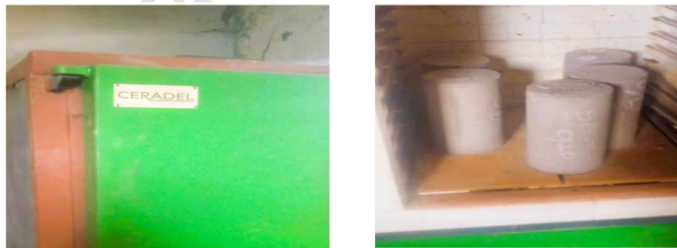
Figure 4: Electric furnace containing the concrete
