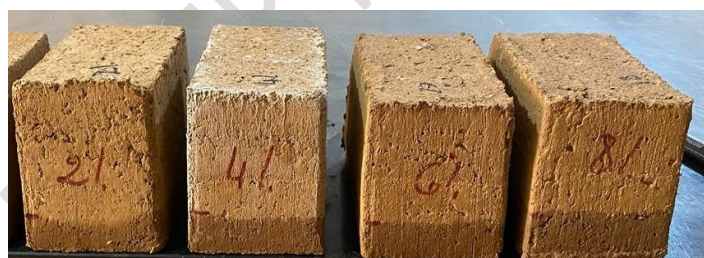
Figure 4: Composite samples after capillary absorption testing
