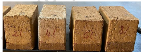
Figure 4: Composite samples after capillary absorption testing
