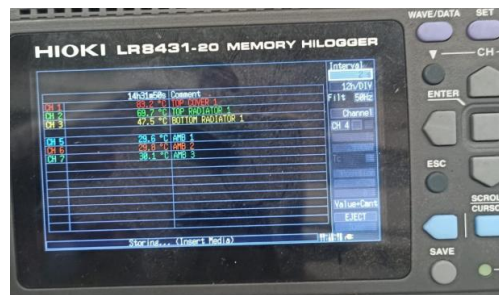
Figure 5. Measurement Results Using a Thermometer Logger
