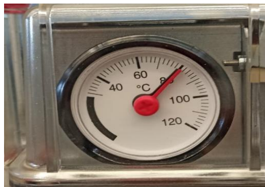
Figure 6. Measurement Results Using a Dial Thermometer
