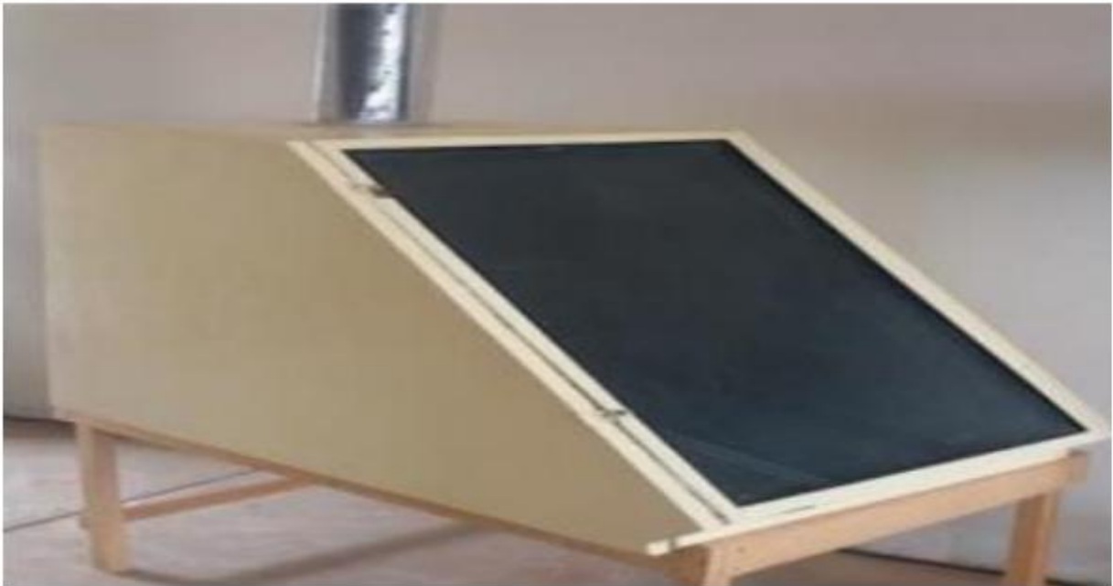
Figure 2. Indirect Natural Convection Solar Dryer
