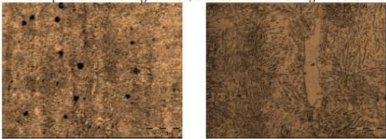
Precipitation hardening TH1050, after solution annealing at 1050°C
