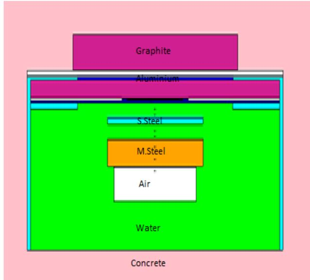
Fig.1. MCNP model for the radial shield of benchmark PCA-REPLICA
