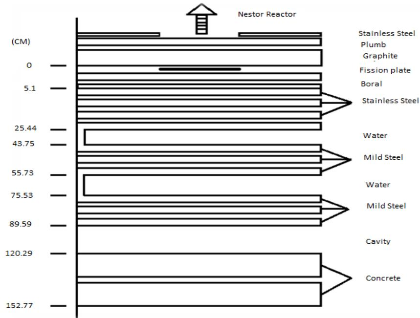
Fig. 3. Radial protection of the NESDIP benchmark experiment
