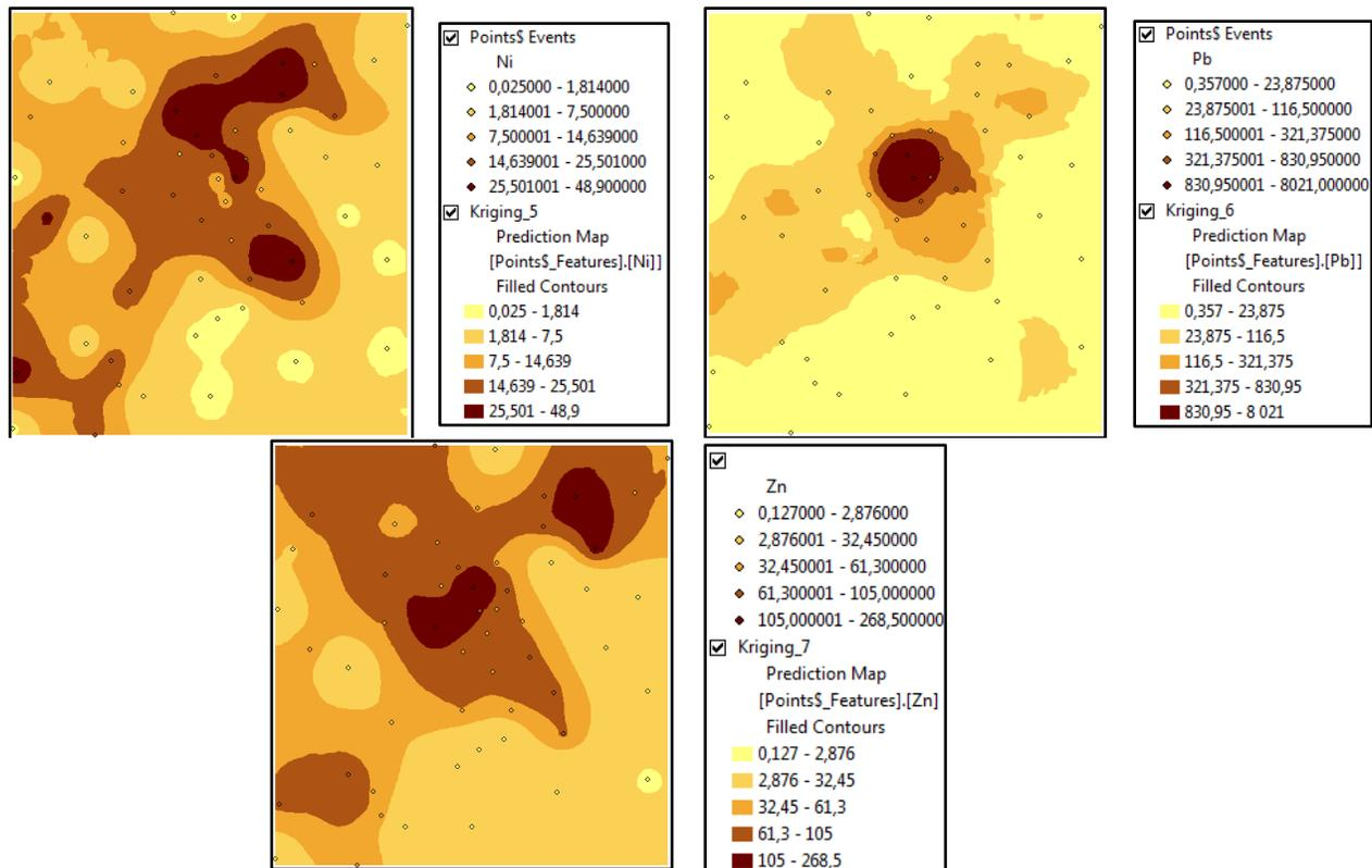
**Figure 4. Spatial distribution maps of Cd, Co, Cr, Cu, Ni, Pb, and Zn concentrations in soils surrounding the tailing pits in the Zaida mine.**
