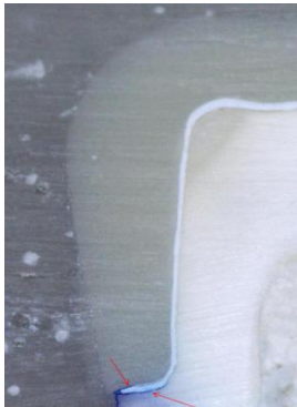
Figure 5 Stereomicroscopic figure: group 3 (Resin based cement-UltraTemp ® REZ) Dye leakage (Red arrows) inside the resin matrix in addition to cement-tooth interface.
