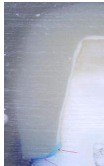
Figure 5 Stereomicroscopic figure: group 3 (Resin based cement-UltraTemp ® REZ) Dye leakage (Red arrows) inside the resin matrix in addition to cement-tooth interface.
