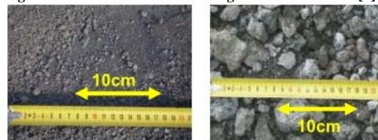
Fig. 1 Fractions of blast furnace slag 0/8 mm a 0/32 mm [4]
