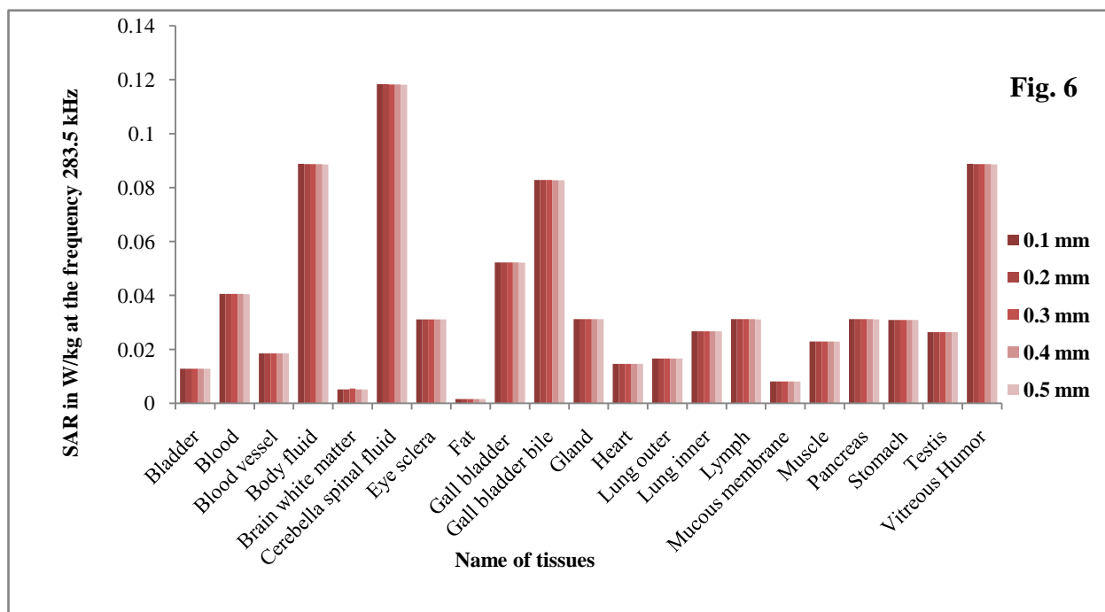
Fig. 6 represents the variation of specific absorption rate (SAR) with respect to different selected tissues of body due to 283.5 kHz of electromagnetic wave
