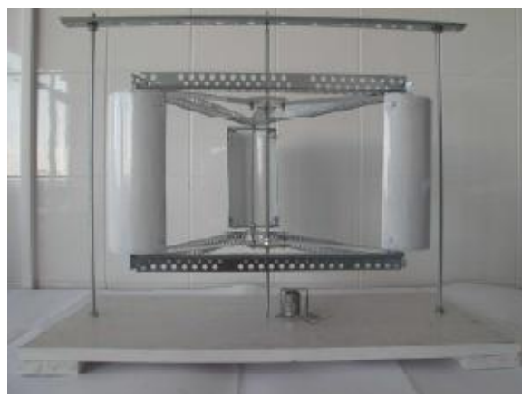
FIG. 5. Experimental-demonstrational model of the wind turbine with vertical semicylindrical blades
