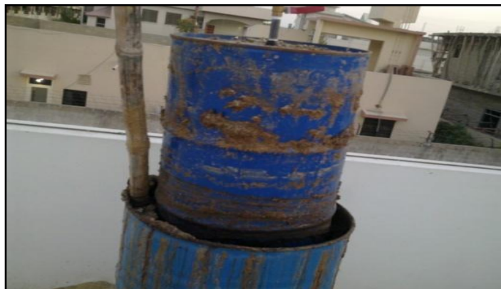
Figure 4 Digester with biogas
