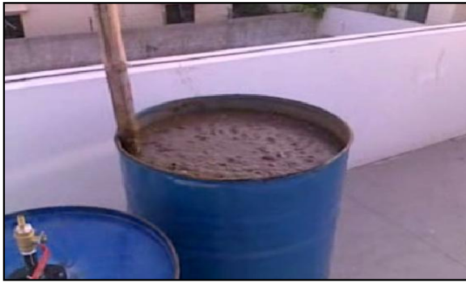
Figure 3 Digester with biomass
