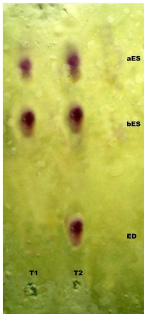
Fig. 1 Screening of endosulfan from Gossypium arboreum L rhizosphere soil by TLC. aES – \alpha Endosulfan; bES – \beta Endosulfan; ED – Endosulfan diol; T1 – Standard; T2 – Sample.
