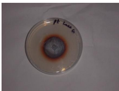
Observation of red colour around a colony with guaiacol indicates laccase activity
