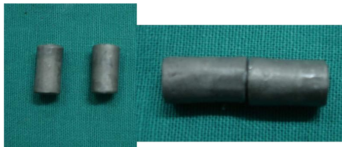
Fig 1: The cast cylindrical alloys and the bonded assembly.
