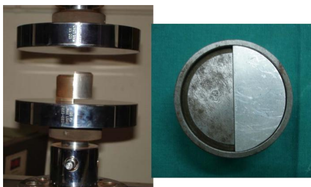
Fig 3: Shear device placed in the Instron testing machine
