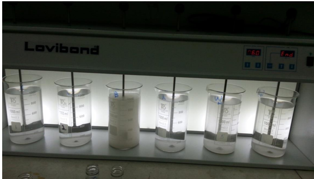
Figure (2):Effect of bioflocculant on the turbidity the preparation of the models after adding the bioflocculant.
