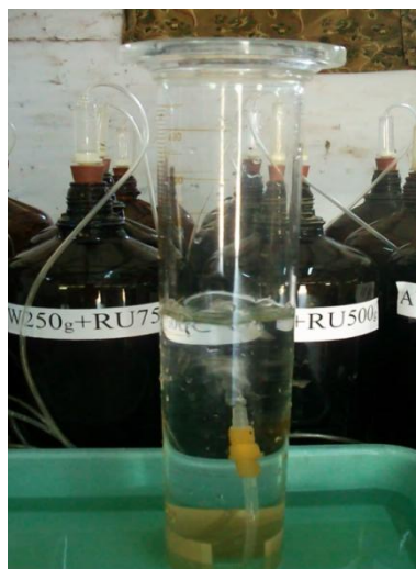
Photo 2 Measurement of gas by water displacement method
