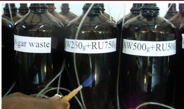
Photo 3 Burning Test of biogas
