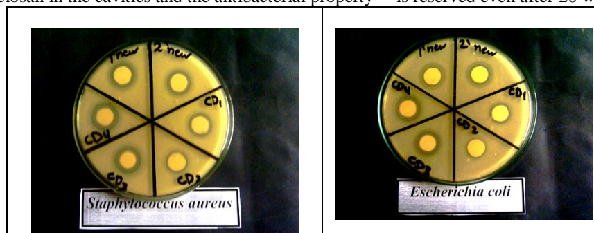
Figure 6 : Effect of \beta - cyclodextrin concentration in presence of glyoxal on the antibacterial properties of cotton fabric reacted with 10g/L triclosan, M:L 1:10(owf)
