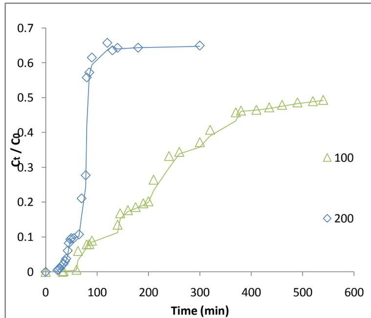
**Fig 3.** Breakthrough curve for adsorption of MG by AAS at different solution flow rates.
