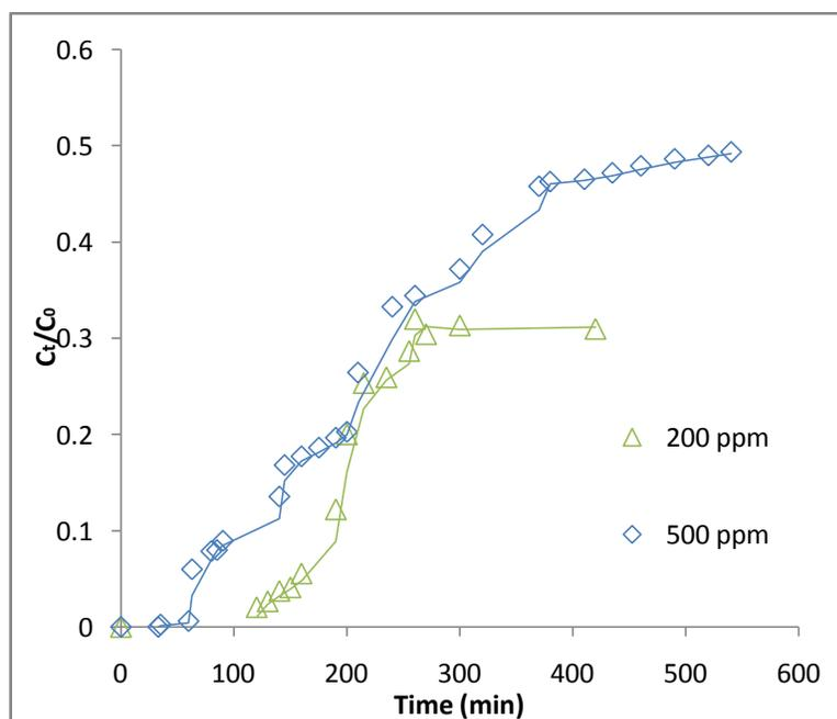
**Fig 2. Breakthrough curve for adsorption of MG by AAS at different initial MG concentrations.**
