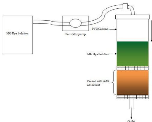
**Fig 1. Continuous column bed Diagram**
