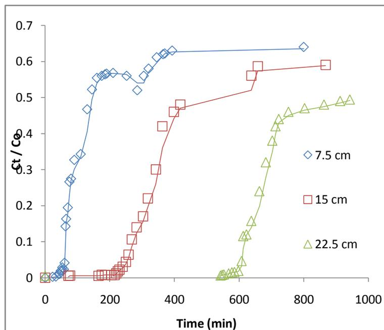
**Fig 4.** Breakthrough curve for adsorption of MG by AAS at different bed heights.
