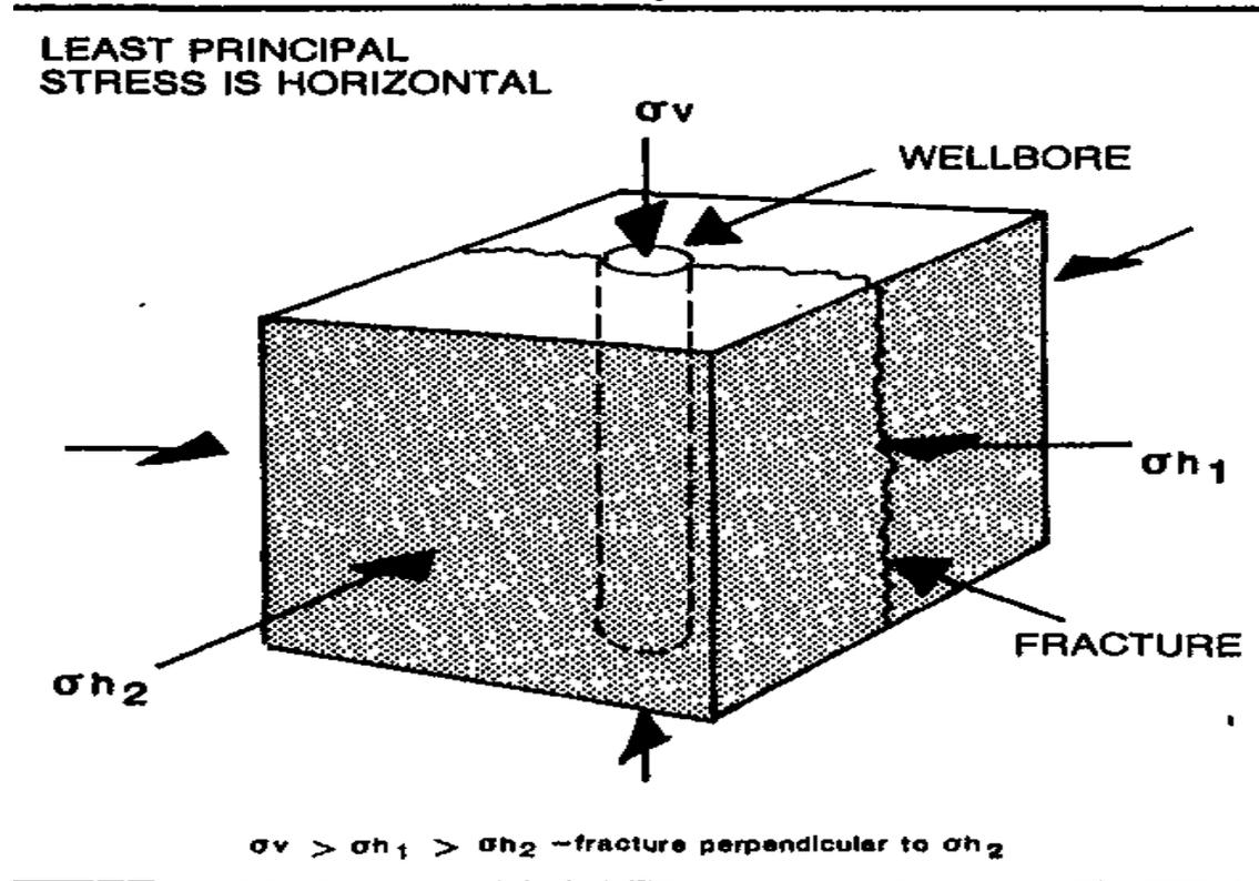
Fig 2: Fracture orientation when the lowest principal stress is horizontal (Guerard Bill).
