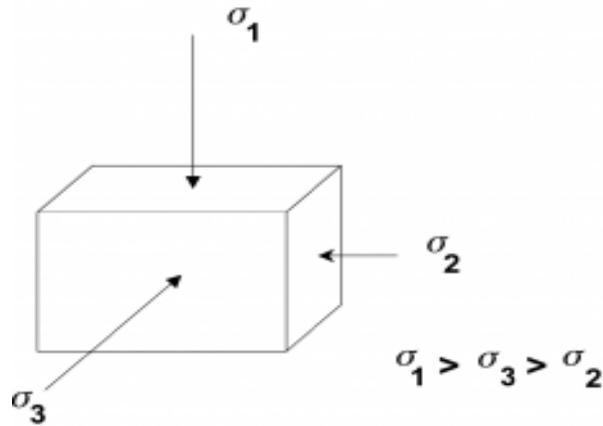
Figure 1: In situ principal stress distribution in a rock
