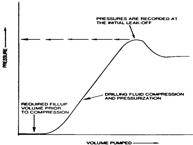
Figure 3: Typical results from a leak-off test
