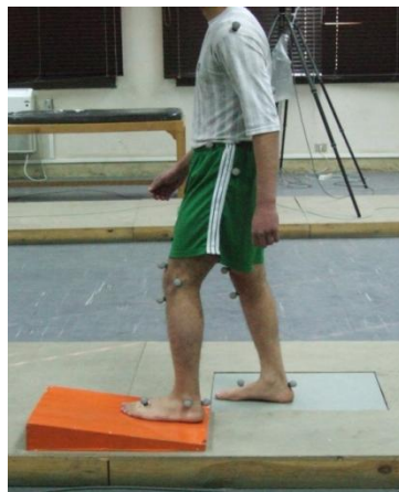
Fig. 42: The second position with 10 degree walking ramp being used.
