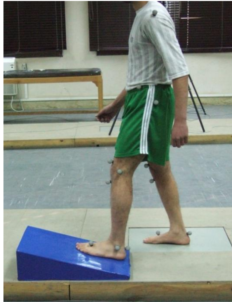
Fig. 43: The second position with 15 degree walking ramp being used.
