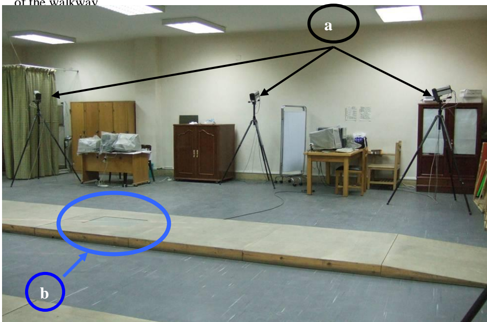
Fig. 33: Placement of the cameras in relation to the force platform. (a) The cameras' placement. (b) The position of the forceplate in the centre of the walkway.
