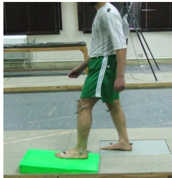
Fig. 41: The second position with 5 degree walking ramp being used.
