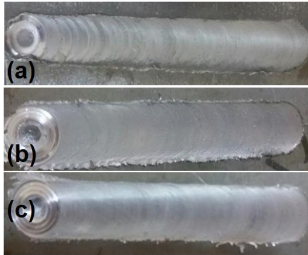
Figure(4) : Appearance of welding using tapered cylindrical threaded pin (TCT) at different rotation speed (a)450RPM,(b)560RPM and (c) 900RPM.
