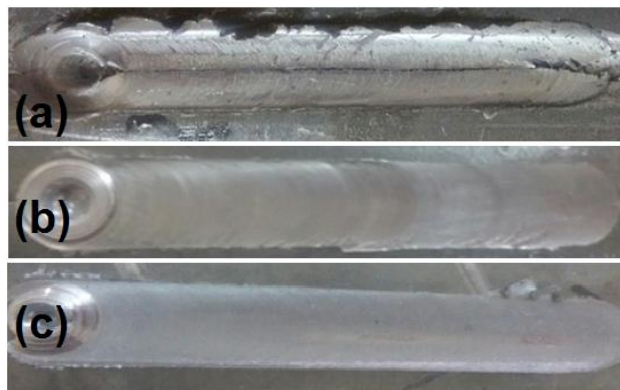
Figure (5) : Appearance of welding using triangular threaded pin (TT) at different rotation speed (a) at450RPM(b)560RPM and (c) 900RPM .
